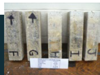
Hycrete prisms after 18 months of exposure
