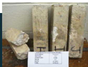
Control prisms after 18 months of exposure
