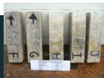
Hycrete prisms after 18 months of exposure
