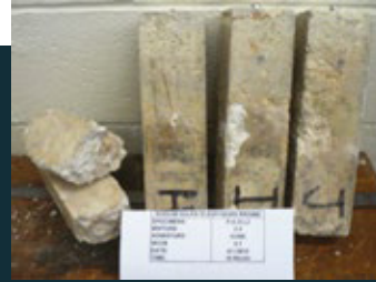
Control prisms after 18 months of exposure
