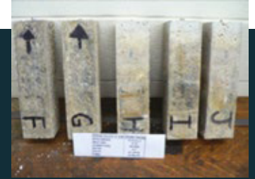
Hycrete prisms after 18 months of exposure
