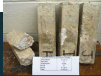
Control prisms after 18 months of exposure
