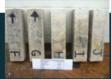
Hycrete prisms after 18 months of exposure
