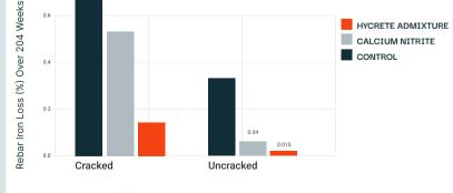
Hycrete effectively reduces rust even in cracked concrete.
