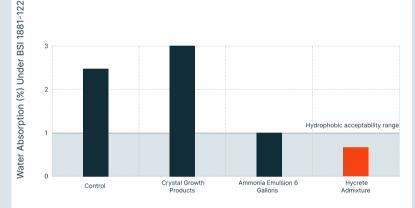
South Carolina Independent Lab Testing: 40/60 Structural Mix, 0.40 W/C 611 Type I-II Cement Polycarboxylate Superplasticizer
