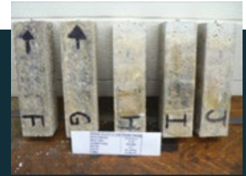
Hycrete prisms after 18 months of exposure
