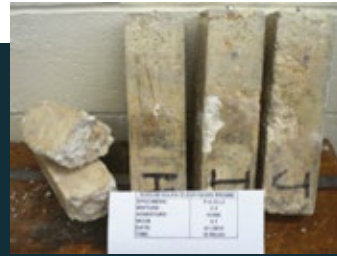
Control prisms after 18 months of exposure
