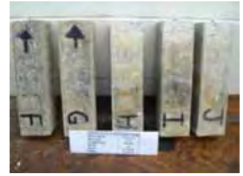
Hycrete prisms after 18 months of exposure
