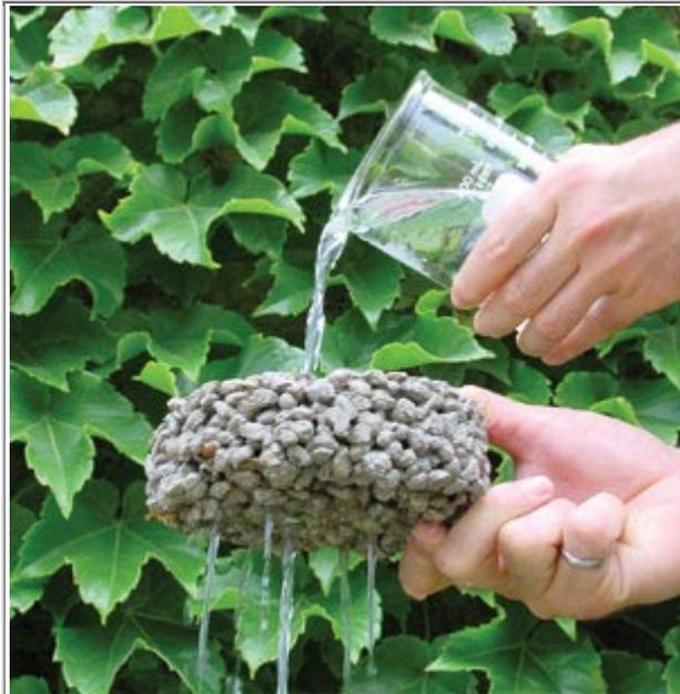
*With pervious concrete, water flows through the concrete and into pervious site surfaces instead of running off impervious surfaces to stormwater sewers. (Image courtesy CTLGroup)*
