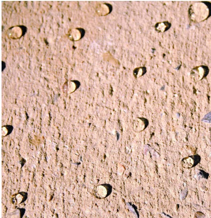
■ Hycrete has corrected the most fundamental flaw in concrete by developing technology to waterproof it
